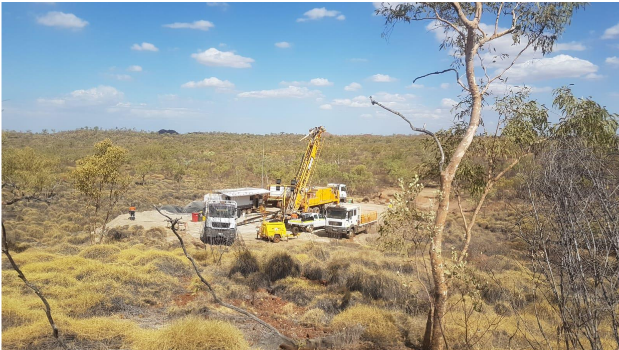
Figure 4 | DDH1 diamond rig and support gear on FNDD001 drill site
